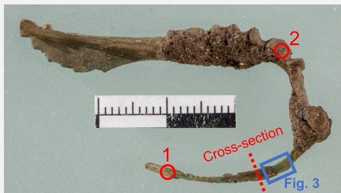
Fig. 2: Location of XRF analyses (red circles), Fig. 3 (documentation of corrosion structure (blue square)) and sampling for cross-section,
