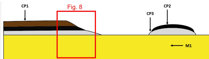
Fig. 7: Stratigraphic representation of the corrosion structure of the sickle by macroscopic and binocular observation with indication of the corrosion structure used to build the MiCorr stratigraphy of Fig. 8 (red square),
