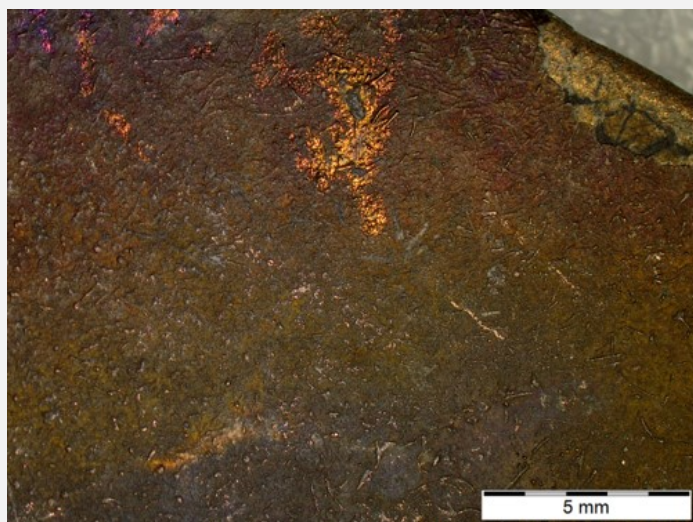
Fig. 4: Brown-yellow and dark-grey corrosion products (detail) of the middle of the sickle,
