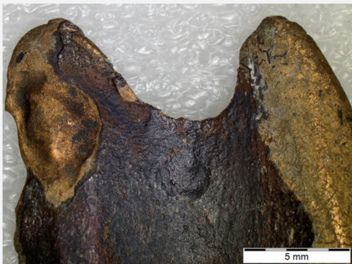
Fig. 2: Brown-yellow and dark-grey corrosion products and lacunas of the corrosion layers (detail) of the haft of the sickle,
