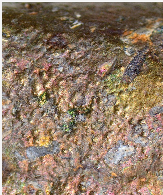
Fig. 2: Dense and brown-yellow corrosion product (detail) of the tang fragment of a knife,
