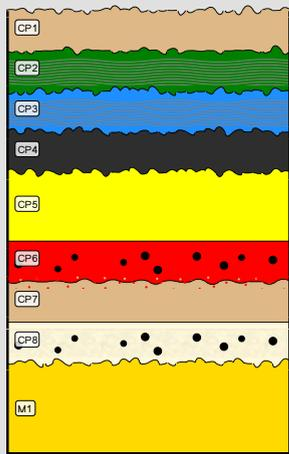
Fig. 6: Stratigraphic representation of the corrosion structure of the tang observed macroscopically under binocular microscope using the MiCorr application with reference to the whole Fig. 5. The characteristics of the strata, such as discontinuity, are accessible by clicking on the drawing that redirects you to the search tool by stratigraphy representation, Credit HE-Arc CR, N.Gutknecht,
