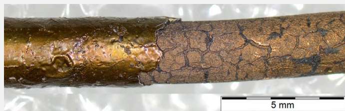
Fig. 3: Dense and smooth olive green corrosion products on the middle of the pin (detail). Discontinuity in the layer is showing the underlying corrosion structure,
