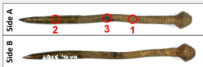
Fig. 5: Sides A and B (opposite sides) of the pin showing the XRF analysis areas (red circles),
