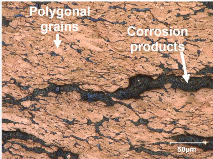
Fig. 9: Micrograph of the metal sample from Fig. 6 (detail), etched, bright field. with polygonal microstructure and presence of longitudinal crack filled with corrosion products,
