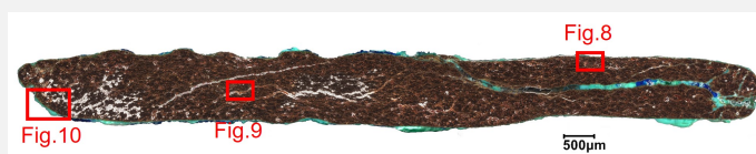
Fig. 6: Micrograph of the cross-section of the sample taken from the coin (Fig. 2) in dark field showing the location of Figs. 8 to 10,
