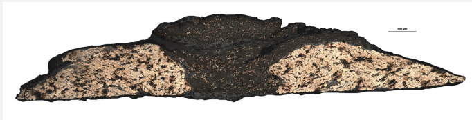
Fig. 8: Micrograph (similar to Fig. 7) of the cross-section of the sample taken from the coin (Fig.2) in bright field after chemical etching,
