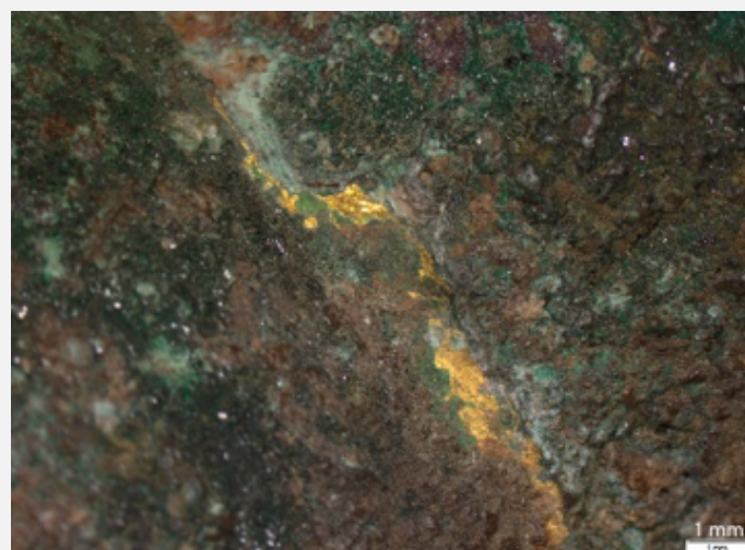
Fig. 3: Remains of foil-gilding on the corroded surface,
