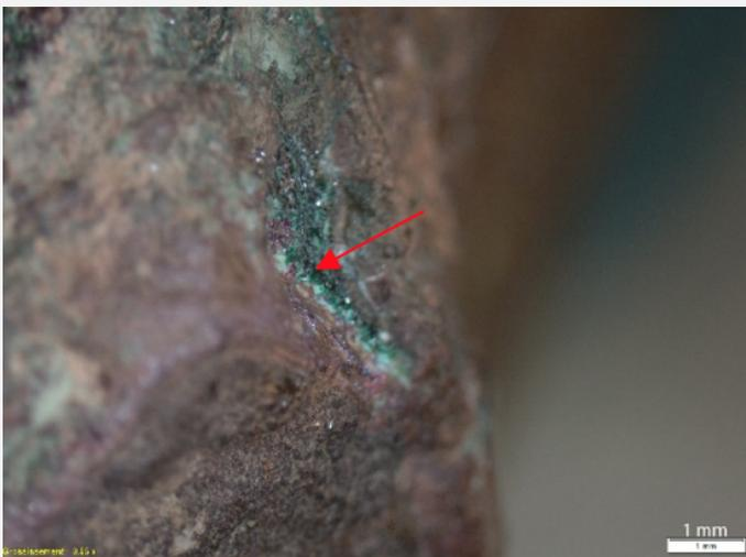
Fig. 13: Observation of the dark green corrosion product,
