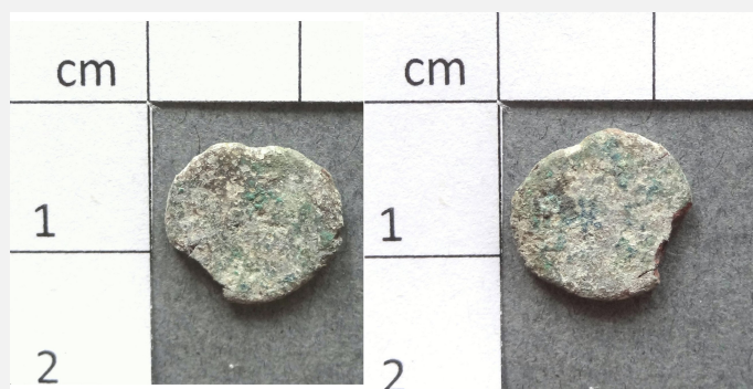
Fig. 1: Views of both sides of a coin from the "Peney hoard" with white, green and blue corrosion products,
