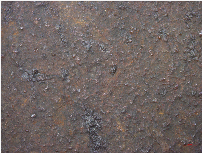
Fig.5: Micrograph of corrosion layer on the front side of the painting,
