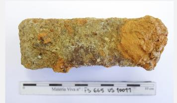
corrosion products (side view),
