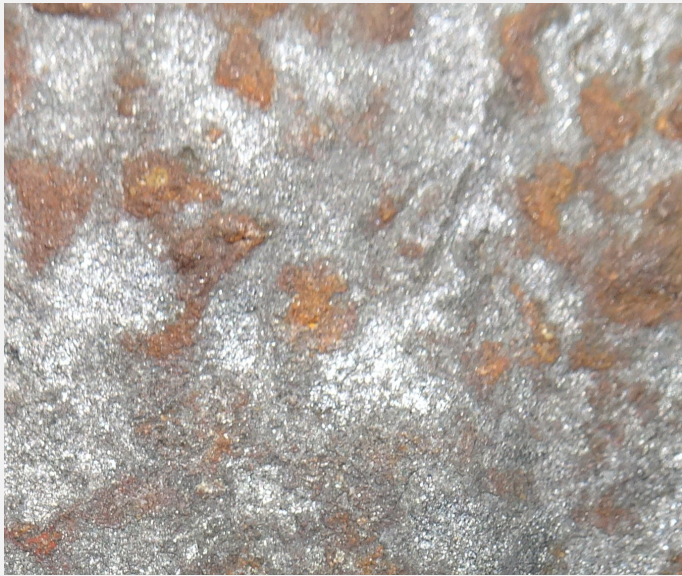
Fig. 4: Detail of the cleaned surface showing shiny grey/blue surface and red/brown spots,
