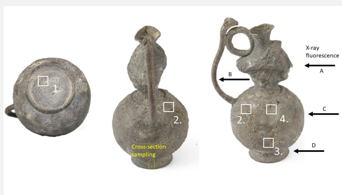
Fig. 2: Locations of the four points analysed with X-ray fluorescence (black arrows A-D), the four samples (numbers 1-4) and the cross-section (yellow) analysed with SEM-EDS,
