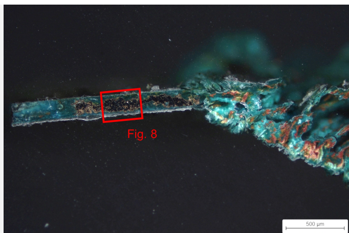
Fig. 6: Micrograph of the cross-section of a sample taken from the fragments of the base of the cup (Fig. 3) showing the location of Fig. 8, dark field,
