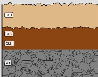
Fig. 12: Stratigraphic representation of the sample taken from the oenochoe base in cross-section (dark field) using the MiCorr application. The characteristics of the strata are only accessible by clicking on the drawing that redirects you to the search tool by stratigraphy representation. This representation can be compared to Fig. 9, Credit HE-Arc CR, C.Degrigny.
