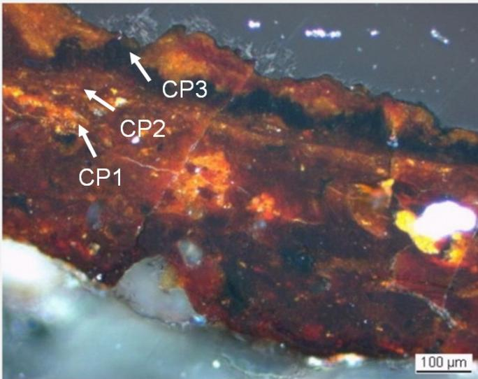
Fig. 12: Micrograph (detail from Fig. 11) corresponding to the stratigraphy of Fig. 14, unetched, polarised light. The black corrosion layer next to the metal surface corresponds to the light-grey layer indicated with an arrow on Fig. 10,
