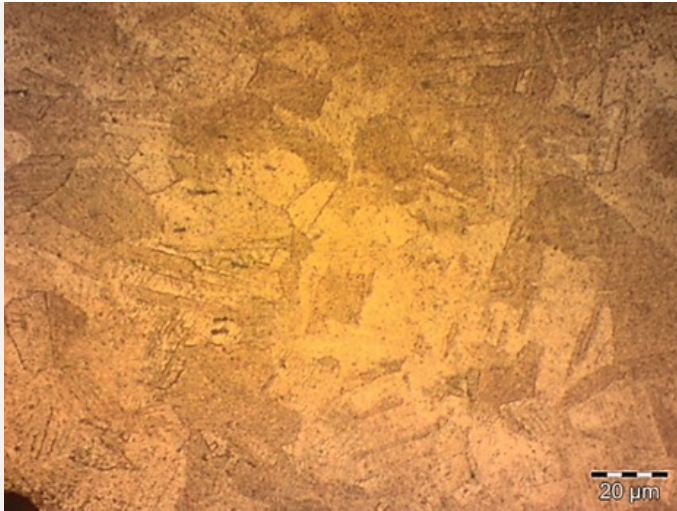
Fig. 7: Micrograph of the selected area of Fig. 6, etched, bright field, 500x. The grains show both twin and strain lines,
