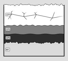
Fig. 4: Stratigraphic representation of the corrosion structure of the lead came observed macroscopically under binocular microscope using the MiCorr application. The characteristics of the strata are only accessible by clicking on the drawing that redirects you to the search tool by stratigraphy representation, Credit HE-Arc CR, A.Gerber.
