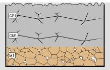
Fig. 10: Stratigraphic representation of the lead came in cross-section (dark field) using the MiCorr application with reference to Fig. 8. The characteristics of the strata are only accessible by clicking on the drawing that redirects you to the search tool by stratigraphy representation, Credit HE-Arc CR, A.Gerber.
