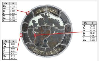
Fig. 6: XRF analyses of a selection of the cames,
