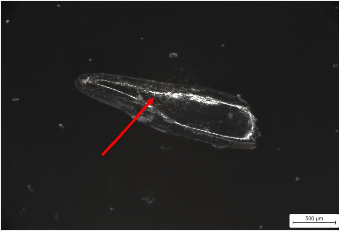
Fig. 7: Micrograph of sample 3 (Fig. 2) of the vase showing a small black element (the red arrow corresponds to the area where EDX analysis was carried out),
