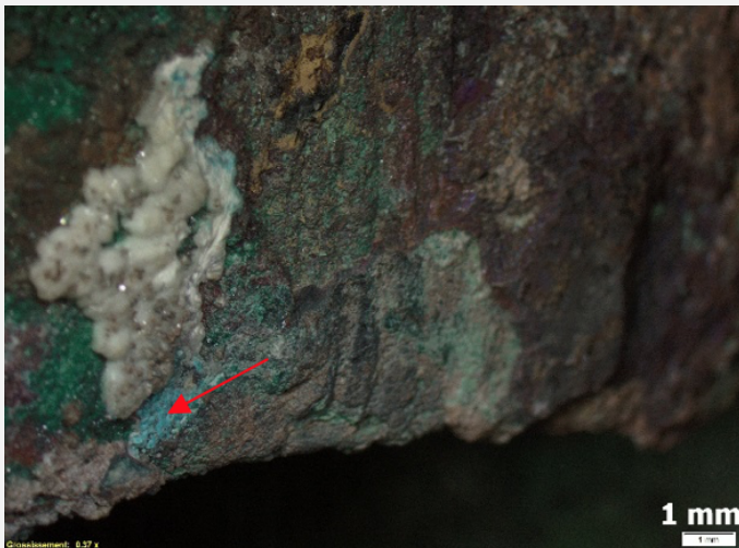
Fig. 17: Observation of the light blue corrosion product,
