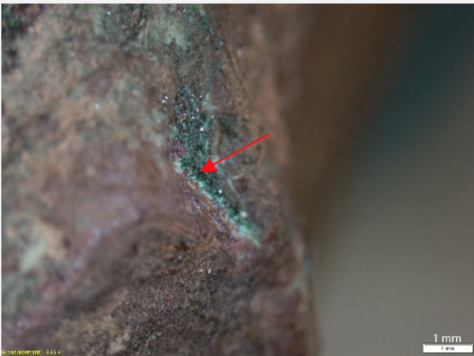
Fig. 13: Observation of the dark green corrosion product,
