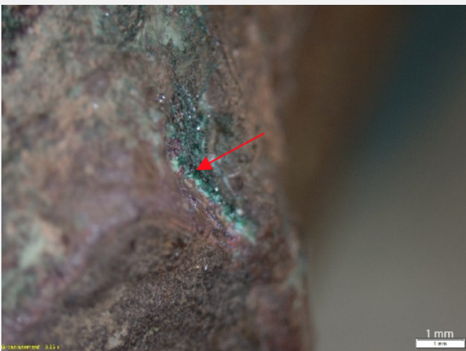
Fig. 13: Observation of the dark green corrosion product,
