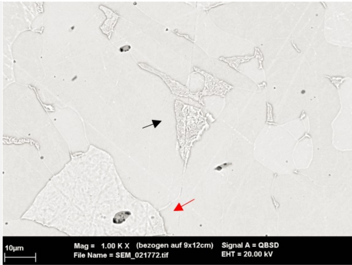
Fig. 7: SEM image of the metal sample from Fig. 3 (detail), BSE-mode, nital etched, bright field. The white ferrite grains contain lamellar pearlite (black arrow) and lenticular grey MnS inclusions (red arrow) in between the grain boundaries,
