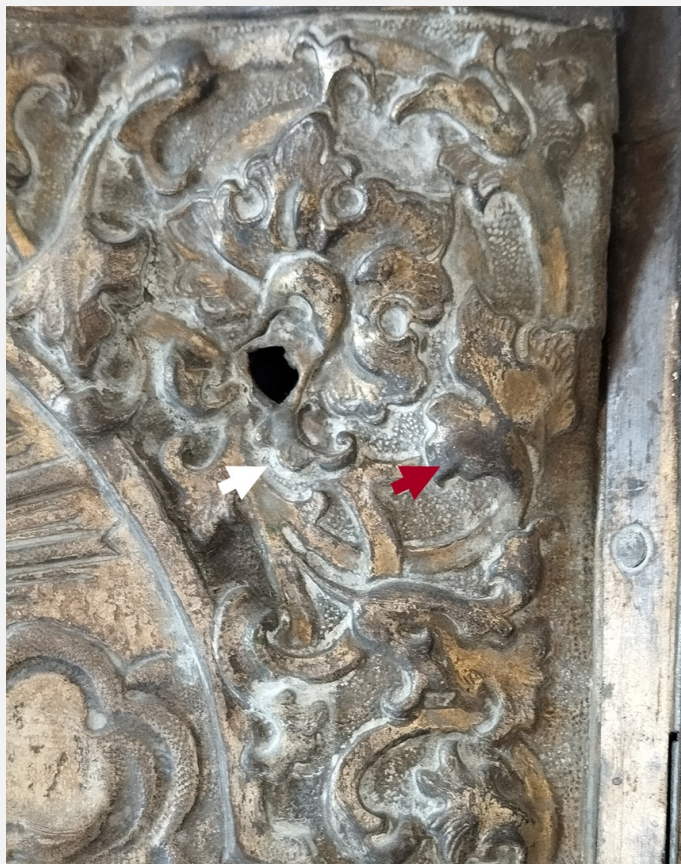
Fig. 2: Location of areas observed: white compound (white arrow) and dark-red (dark-red arrow),
