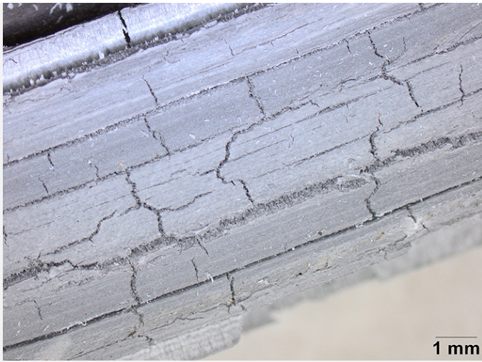
Fig. 3: Detail of the corroded lead came,
