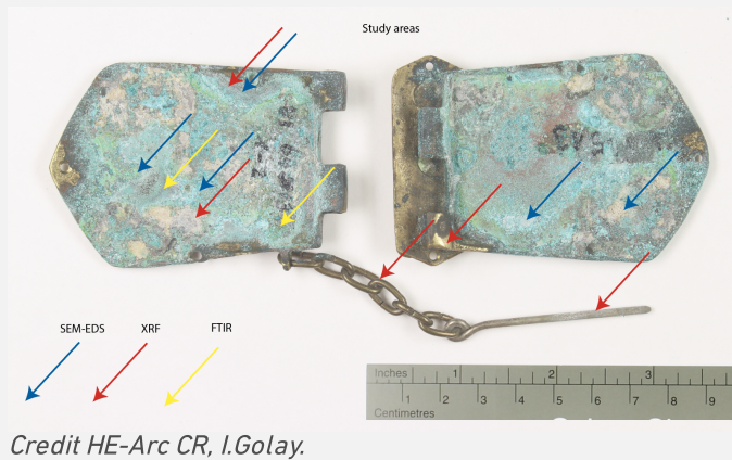
Fig. 4: Location of the study areas on the back face of the belt buckle,
