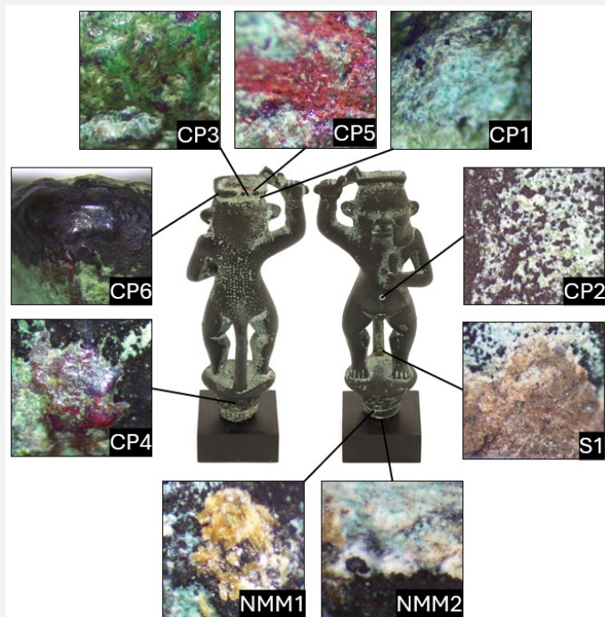
Fig. 4: Details of corrosion forms as observed under binocular microscopy,
