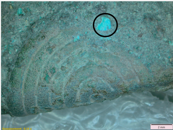
Fig.12: Sample 1 - turquoise powdery corrosion (CP1),
