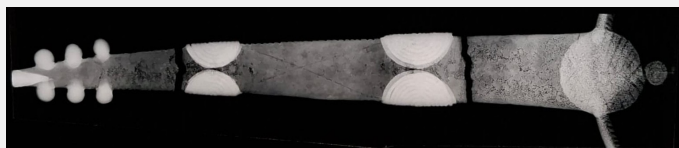
Fig. 14: X-radiography image of the handle of the ladle showing the two fractures,
