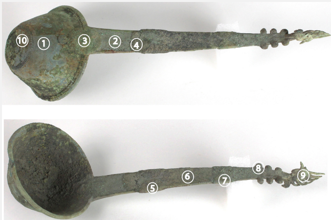
Fig.8 : Location of XRF analyses on the front and rear faces of the handle,
