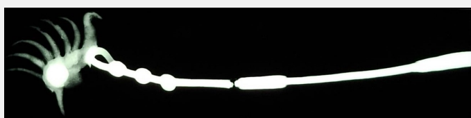
Fig. 15: X-radiography image of the cockerel of the side of the handle showing the top fracture,
