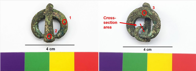
Fig. 2: Location of study areas for XRF analysis (red circles) and the sampling area for cross-section (dashed line),
