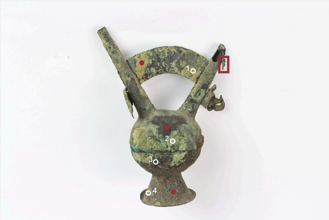
Fig. 2: The funerary flask showing the location of XRF analyses (white points), sampling areas for SEM-EDS (red points) and sampling area for examination on cross-section (red rectangle),
