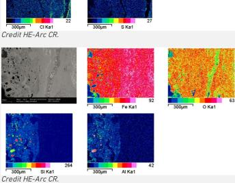
Fig. 13: SEM image, BSD-mode, and elemental chemical distribution of the selected area from Fig. 10 (reversed picture). Method of examination: SEM/EDX, Laboratory of Analytical Chemistry, Empa,
