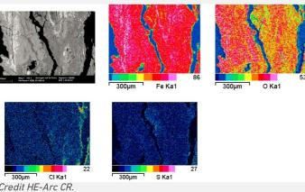
Fig. 12: SEM image, BSD-mode, and elemental chemical distribution of the selected area from Fig. 10 (reversed picture). Method of examination: SEM/EDX, Laboratory of Analytical Chemistry, Empa,
