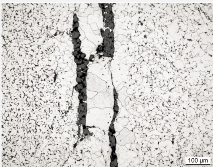
Fig. 8: Micrograph of cross-section from Fig. 3 (detail), nital etched, bright field. We observe a hypoeutectoid steel including a ferritic zone surrounded by slag inclusions,
