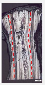
Fig. 7: Micrograph of metal samples 1 and 2, etched with Oberhoffer's reagent, bright field. The P segregation along the welding seams is outlined. The main welding seams are marked by red dotted lines,
