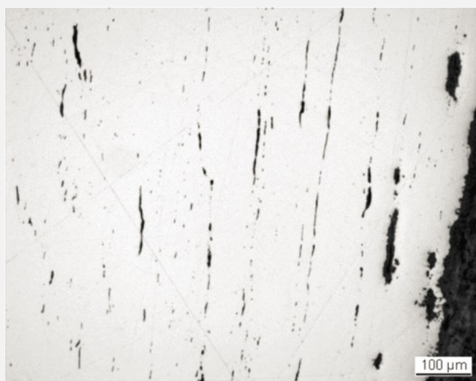
Fig. 4: Micrograph of metal sample 1 from Fig. 3 (reversed picture, detail), unetched, bright field. Slag inclusions organized in rows mark the welding seams,
