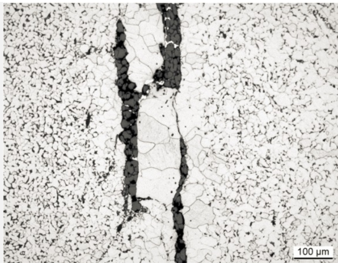
Fig. 8: Micrograph of cross-section from Fig. 3 (detail), nital etched, bright field. We observe a hypoeutectoid steel including a ferritic zone surrounded by slag inclusions,
