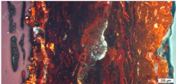
Fig. 11: Micrograph (same as Fig. 10), unetched, polarised light. From left to right: the metal in violet, the successive corrosion layers having a grey or an orange to red colour. The outer layer is orange-brown with quartz inclusions in white,
