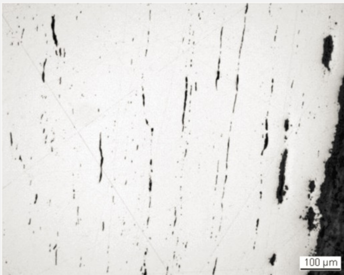
Fig. 4: Micrograph of metal sample 1 from Fig. 3 (reversed picture, detail), unetched, bright field. Slag inclusions organized in rows mark the welding seams,
