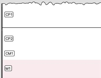
Fig. 5: Stratigraphic representation of the object in cross-section using the MiCorr application. This representation can be compared to Fig. 11.
