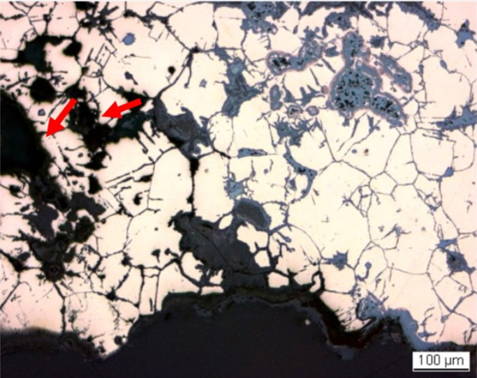
Fig. 4: Micrograph of the metal sample from Fig. 3 (detail), unetched, bright field. Extensive inter- and transgranular corrosion has developed within the metal. Large pores are visible (arrows) inside the remaining metal,
