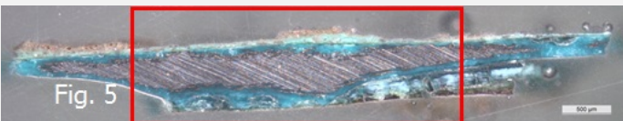
Fig. 4: Micrograph of the cross-section showing the location of Fig. 5. Unetched, dark field, 50x,
