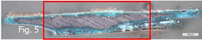
Fig. 4: Micrograph of the cross-section showing the location of Fig. 5. Unetched, dark field, 50x,
