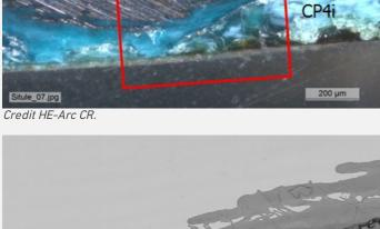
Fig. 9: SEM image, BSD-mode of the metal sample from Fig. 8 (detail) showing cleavage between the inner blue (CP5i) and green (CP4i) lavers.
