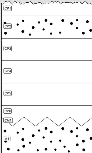
Fig. 4: Stratigraphic representation of the object in cross-section using the MiCorr application. This representation can be compared to Fig. 8.
