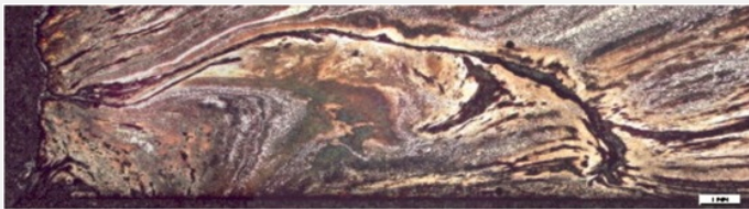
Fig. 5: Micrograph of the metal sample from Fig. 3 (reversed picture, detail), etched with Oberhoffer's reagent, bright field. The etching shows the P segregation near the welding line and outlines the irregular P distribution in the metal (white P-rich areas, dark P-poor areas),
