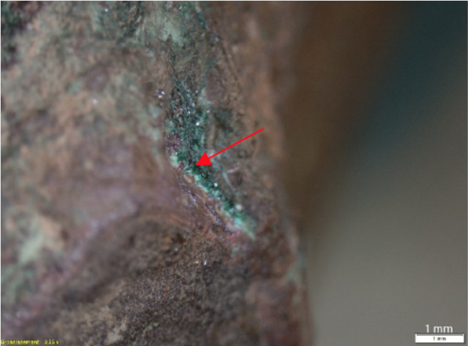
Fig. 13: Observation of the dark green corrosion product,
