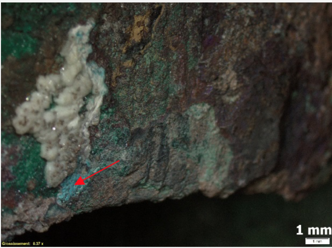
Fig. 17: Observation of the light blue corrosion product,
