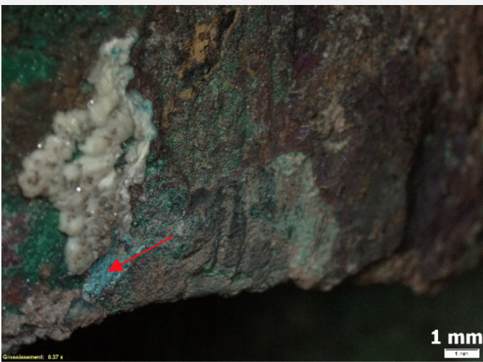
Fig. 17: Observation of the light blue corrosion product,
