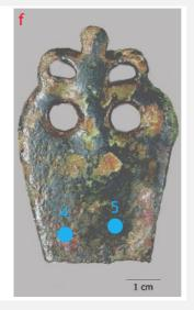
Fig. 2: Cooking pot handle after treatment: front (e) and back (f). Location of sampling for SEM-EDS, Raman (yellow square 1), XRD analyses (yellow square 1 and 2), as well as the location of the XRF analyses (blue points 3, 4, 5),
