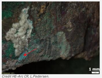
Fig. 17: Observation of the light blue corrosion product,
