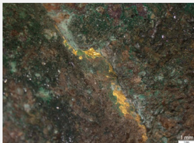
Fig. 3: Remains of foil-gilding on the corroded surface,
