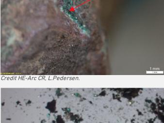
Fig. 14: Dark green corrosion product identified as paratacamite, atacamite Cu2Cl(OH)3 by XRD. Microscopic examination under polarized light,
