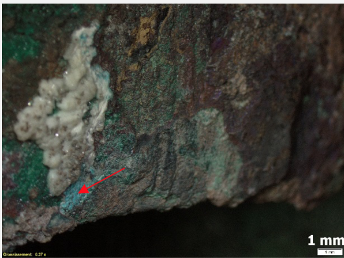
Fig. 17: Observation of the light blue corrosion product,
