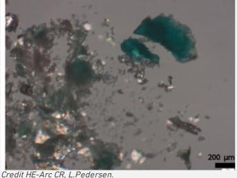
Fig. 18: Light blue corrosion product identified as chalconatronite Na2Cu(CO3)2·3H2O by XRD. Microscopic examination under polarized light,
