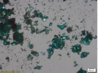
Fig. 16: Light green corrosion product identified as paratacamite, atacamite (Cu2Cl(OH)3) by XRD. Microscopic examination under polarized light,
