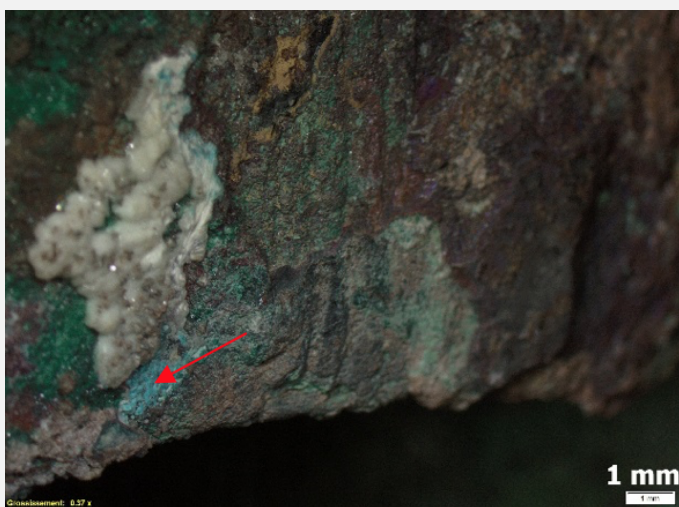
Fig. 17: Observation of the light blue corrosion product,
