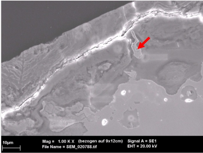
Fig. 7: SEM image (detail of Fig. 5, reversed picture), SE-mode. From bottom right to top left: the metal, the inner and outer corrosion layers separated by a large fissure. The red arrow indicates a remnant of the Sn-rich alpha-delta eutectoid,
