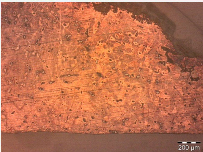
Fig. 8: Micrograph of the metal sample from Fig. 4 showing a dendritic structure and grains,
