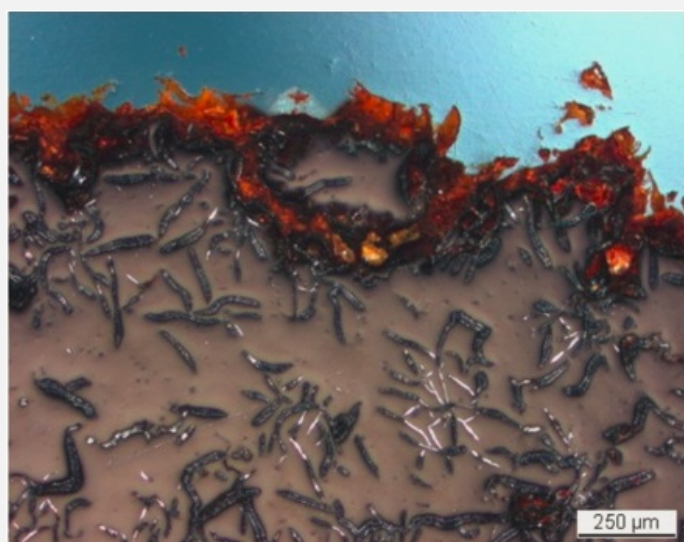
Fig. 10: Micrograph (same as Fig. 9) corresponding to the stratigraphy of Fig. 4, unetched, polarised light. We observe in violet the metal, in orange the corrosion, in blue the resin,
