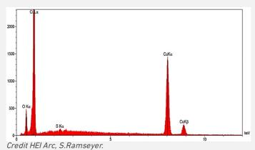
Fig. 14: EDS spectrum of sample 2 (red particle),
