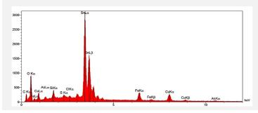
Fig, 12: EDS spectrum of sample 1 (yellow powder),
