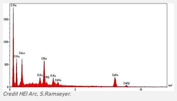
Fig. 16: EDS spectrum of sample 4 (white particle),
