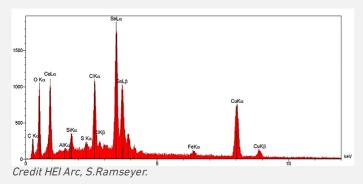
Fig. 15: EDS spectrum of sample 3 (green corrosion product),
