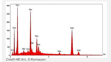
Fig. 13: EDS spectrum of sample 2 (green particle),
