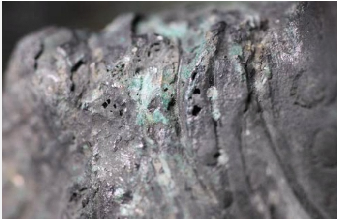
Fig. 4: Porous zone located on Fig. 2 (blue square),
