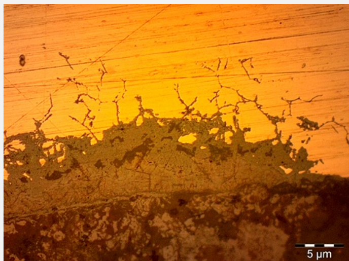
Fig. 9: Micrograph of the metal sample from Fig. 4, unetched, bright field, 50x. The grain boundaries are revealed by the intergranular corrosion,
