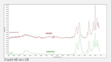
Fig. 15: FTIR spectrum (ATR mode) of the outer green layer compared to the malachite standard spectrum. Method of analysis: FTIR spectroscopy, HE-Arc CR.,
