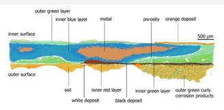
Strata Composition Soil (S) Ca, Si, Al, Fe Black deposit (D1) Orange deposit (D2) Ferrous oxides White deposit (D3) Ca Outer green curly corrosion product (CP1e) Copper carbonates (curly malachite) Copper oxide (cuprite ?) Inner red (CP2i) Outer green layer (CP3i) Copper carbonates (malachite) Copper carbonates (?) + Sn Copper carbonates (?) + Sn Inner green layer (CP4i) Inner blue layer (CP5i) Remnant metal phase (M) Bronze (90%Cu, 10% Sn)
