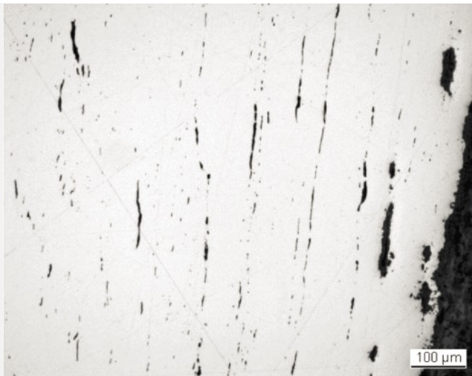
Fig. 5: Micrograph of metal sample 1 from Fig. 3 (reversed picture, detail), unetched, bright field. Slag inclusions organized in rows mark the welding seams,
