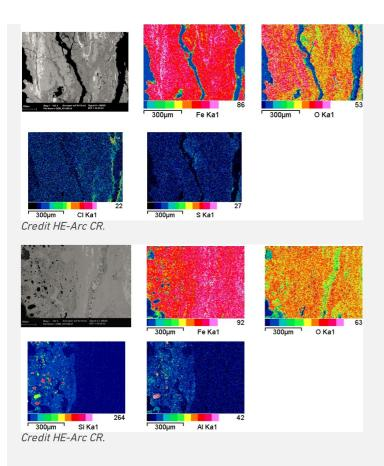
Fig. 14: SEM image, BSE-mode, and elemental chemical distribution of the selected area from Fig. 10 (reversed picture). Method of examination: SEM/EDS, Laboratory of Analytical Chemistry, Empa,
