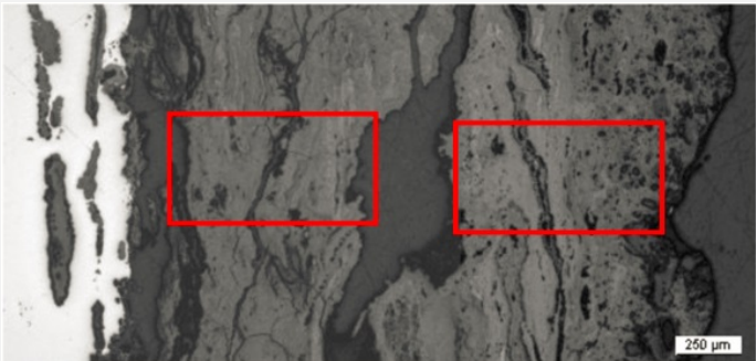
Fig. 11: Micrograph showing the metal - corrosion crust interface from Fig. 3 (reversed picture, detail), unetched, bright field. The micrographs of Fig. 13 (left) and Fig. 14 (right) are marked by rectangles,
