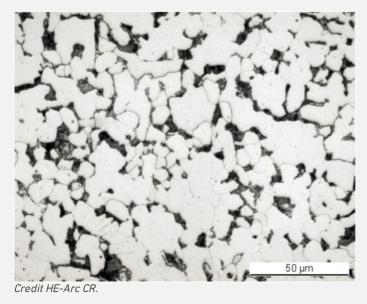
Fig. 10: Micrograph of metal sample 2 from Fig. 3 (detail), nital etched, bright field. We observe a hypoeutectoid steel with a structure of ferrite in white and pearlite in black,
